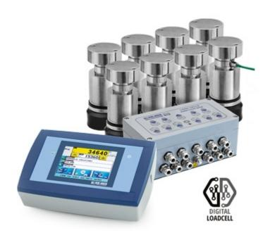
Digital weighbridges kit made up of 3590ETD touch screen weight indicator with AF03 software for weighbridges, 8 stainless steel IP68 "RCPTD" digital load cells, complete with galvanized steel oscillating resting joints and digital equalisation box, with surge arresters.
