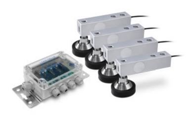
Ideal for creating platforms with 4 load cells of various sizes and capacities. The kit is made up of 4 350 Ohm IP67 nikel-plated load cells, OIML and NTEP approved, together with adjustable resting feet and an equalisation box.
