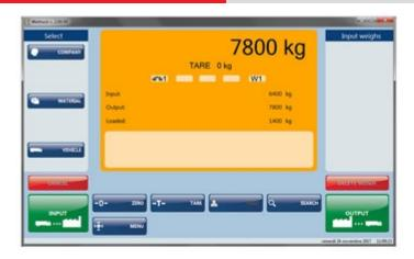
Software for a PC which allows to completely manage a weighbridge system, combinable to the DFW, DGT and 3590 series' weight indicators. Besides the complete management of the connected scale, the programme offers a simple and intuitive operator interface, databases for the storage of the customer, material, and vehicle data, management of the totals and programmable printouts.
