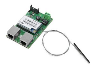
Small sized WIFI board for a connection inside the indicator with provided cable. The sticky antenna can be applied on the case and allows connecting any scale or weighing system to the corporate network.
