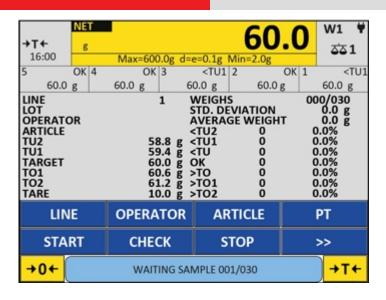
Specific software for production checking which includes all the main check functions, either in sample statistic mode or in complete statistic mode (as provided for by the directive N. 76/211 /EEC). The touch screen interface shows in real time, every statistical data field with a chart or a numerical form. The simultaneous production lines check function allows up to 10 contemporaneous different articles check. CE-M approvable (OIML R-76 / EN 45501).
