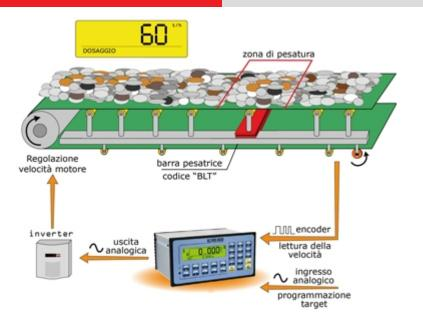
Software version for the measurement/integration of the weight, flow of material transitioning on the weighing belt, with memorisation of the quantity of dosed material; possibility of adjusting the flow through the 16 bit analogue output and PID control. Possibility of remote management of the instrument, through Sysway or Modbus RTU protocols, or Profibus through external optional interface.
