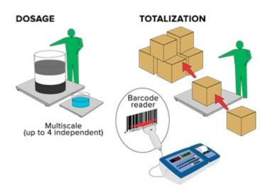
Suitable for advanced applications of weight totalization and formula weighing, with data, database and print management. CE-M approvable (OIML R-76 / EN 45501).
