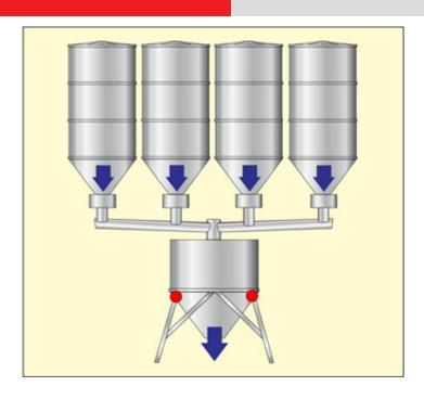
Configuration which allows the dosage of various products, in loading or unloading, as well as mixing and formulation, with the possibility of managing mixers, burners or vibrators using dedicated contacts.
