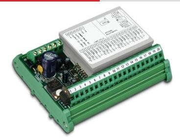
Weight transmitter with 0-20mA, 4-20mA, 0-10Vdc or +/- 5Vdc analogue output at choice. Suitable for assembling on the panel rear or in tin box on omega bar. Normally used with 12-bit analogue / digital cards installed on PLC
