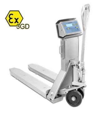
AISI 304 stainless steel pallet truck scale for use in ATEX hazardous areas 2 & 22, with Ex II 3G IIC T6 Gc X and Ex II 3D IIIC T115C° Dc X protection. Also available in approved version for legalfor-trade use.
