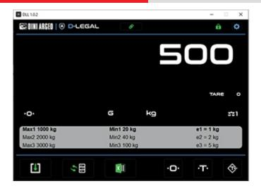
DLEGAL is a program for saving approved weighing operations. It is a real virtual alibi memory, directly on a PC and without storage limits. With this new software, all data is saved in a legal for trade approved file that can be exported to Excel. It is designed to simplify data exchange with external programs using a comprehensive API package.
