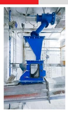
The Master BulkSlide is a solids flow meter that measures with accuracy from ± 0,5 percent. It can be used for most solid bulk products that are free-flowing and non-sticky. The BulkSlide calculates the product flow and total by measuring the force of the bulk product as it contacts the curved plate within the BulkSlide assembly.
