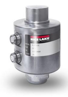
Digital canister load cells for CE-M approved weighbridges, tanks, silos, etc. Manufactured in STAINLESS STEEL, IP68 protection degree, 4000 divisions.
