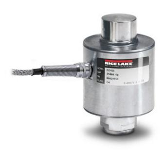
Canister load cells for CE-M approved weighbridges, tanks, silos, etc. Manufactured in STAINLESS STEEL, IP69K protection degree, 4000 divisions.
