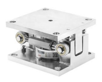
KCP50 is an accessory designed for the correct mounting and operation of CPA and CPX series compression <u>load cells</u> under silos, hoppers and tanks (up to 50t per support point). KCP50 offers a correct protection against overloads and side forces and actively contributes to the protection against accidental tipping of the silo.
