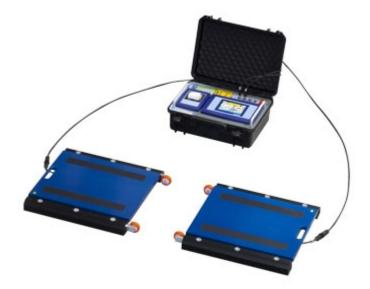
It weighs the vehicle axles and calculates the total weight. Consisting of two WWS series portable pads and the touch screen weighing terminal with integrated printer. Wired version.
