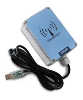
2.4 GHz Radio frequency interface box, for wireless communication between PC/master device and weight indicator/repeater. Up to 39 channels, connection through USB or RS232 port (depending on the model).
