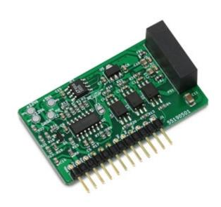
16 bit analogue output, in voltage or in current. Programmable as 0...5/0...10VDC, 0...20/4...20mA through the **indicator** or through the PC with Dinitools. Particularly suitable for use with PLC's and in industrial environments.
