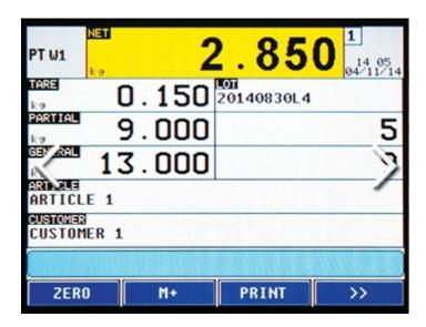
• The PC software "Dini Display Tool" allows for the quick customisation of the TOUCH display.
