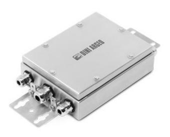
AISI 304 stainless steel junction box with IP68/IP69K protection from water and dust, fitted with electronic board for junction and equalisation of 4 load cells.
