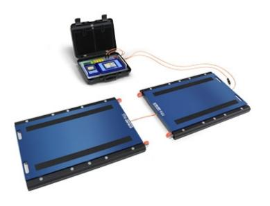
Specific Kit for the manual static weighing of axles. It is composed by two portable wheel weighing pads WWS series and by the touch screen weight indicator 3590ETKR series, with integrated printer. The user interface is clear, simple and intuitive and displays in real time the weight of the axle, the total weight, the tare and the identification code of the vehicle. The ticket reports all the weight data, in order to facilitate registration and traceability.
