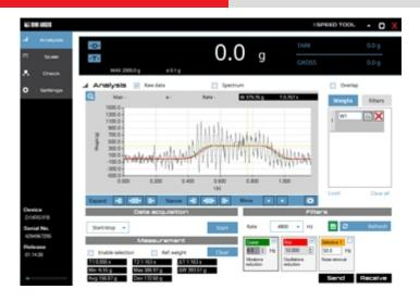
PC software that allows you to record the signal coming from the load cell in real time and process it by applying specific filters to remove vibrations, disturbance and noise. Indispensable to obtain precise and fast weighs in automated weighing systems.
