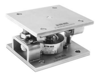
UNI EN 1090 certified mounting kits for compression <u>load cells</u> CPX series up to 12,500kg and CPA up to 10t, suitable for weighing hoppers, silos and large capacity tanks.
