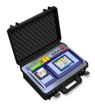
Digital weight indicator with a big touch screen display, suitable for the weighing of vehicles, planes and objects with multiple points of support. It allows the visualization of all the weighing data and the customization of the screens, simplifying the user operations. Fitted with 3 serial ports, transmission protocols for data communication, completely configurable printouts, integrated alibi memory, and port for connection to barcode/badge reader. CE-M approvable (OIML R-76 / EN 45501).
