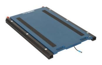
Pads designed for creating weighing stations for large sized vehicles fitted with twinned wheels or large sized tyres (articulated lorries, tractortrailers, building yard vehicles, etc.); fitted with integrated wheels for easing the transport. Particularly suitable for dynamic weighing.
