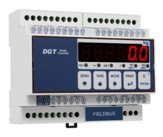
4-channel weight transmitter for weight transfer to PLC via fieldbus, analog output or RS485. It allows the reading and diagnostics of each load cell or each connected scale (up to 4).
