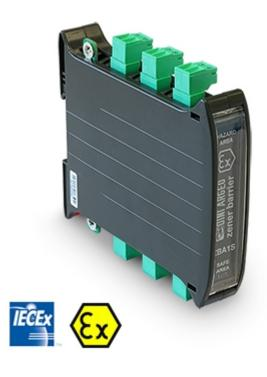
The Zener Barrier ZBA1S is the perfect solution for the connection between a weighing terminal and a weight receiver system in the ATEX ZONE. ZBA1S integrates three barriers in one, protecting the excitation line, signal and sense. This feature makes the installation easier, especially in small spaces. This saves time and money.
