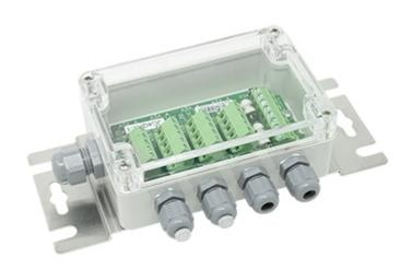
Simple junction box with IP67 protection and 4 inputs equipped with electronic board for junction of the signals of 2, 3 or 4 load cells. Screw terminal boards to facilitate the connection. The protection circuit protects against lightning and overvoltage. The reduced costs make it the ideal choice for static weighing systems such as silos, tanks and big containers.
