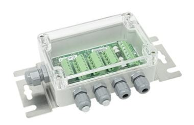
Junction box with 4 inputs and protection IP67 suitable for outdoor environments. It can be used as equalization or simple junction box of 2, 3 or 4 load cells. Screw terminal boards to facilitate the connection and signal adjustment trimmer, for an accurate and reliable equalization. The protection circuit protects from lightning and overvoltage.
