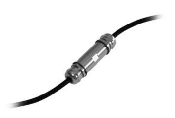
Stainless steel junction box with IP68 protection from water and dust, equipped with electronic board to join 2 load cell cable sections. The 8 screw terminal boards facilitate the cable connection. The stainless steel body ensures solidity and durability.
