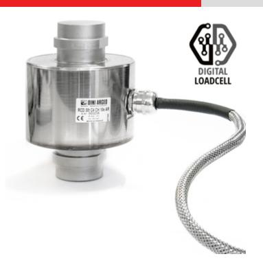
Digital version of compression load cells, 4000 divisions, ideal for CE-M approved weighbridges, tanks, silos, etc. Manufactured in STAINLESS STEEL, with IP68 protection, fitted with "anti rat" armoured cable.
