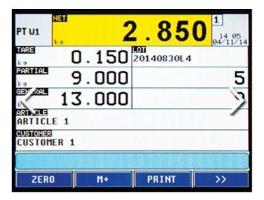
• The "Dini Display Tool" is a PC software which allows you to quickly customize the TOUCH SCREEN.
