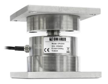
Thanks to the ELGO modular kit, it is possible to quickly install CPX compression <u>load cells</u>, up to 12.500kg for weighing of silos, tanks, or different kinds of structures, containing installation costs. Built in STAINLESS steel and extremely simple to clean, ELGO is ideal for weighing in environments which are hostile, or that have high hygiene requirements. ATEX certification II 2GD c IIC T6 85°C.
