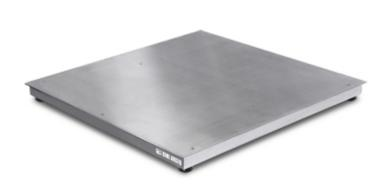
Electronic STAINLESS STEEL AISI 304 weighing low profile platforms with removable loading plate fitted with IP68 STAINLESS STEEL C6 approved <u>load cells</u>. Suitable for creating scales and electronic weighing systems for all types of industrial and commercial applications. Available in high resolution and suitable for ATEX zones.
