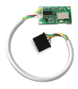
Thanks to the Bluetooth <u>interface</u>, the exchange of data between the digital scales and the computer system will be simpler and quicker: it is sufficient to be at a few meters from the weight indicator in order to update the databases, read the memory, transmit commands, receive data, check the configuration, etc.
