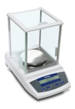
High performance analytical scale, compact and versatile, fitted with windscreen. Suitable for laboratories, pharmacy and industrial applications.
