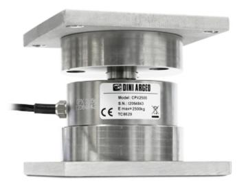
Thanks to the ELGO modular kit, it is possible to quickly install CP/CPX compression <u>load cells</u>, up to 12.500kg, for weighing of silos, tanks, or different kinds of structures, containing installation costs. Built in STAINLESS steel and extremely simple to clean, ELGO is ideal for weighing in environments which are hostile, or that have high hygiene requirements. ATEX certification II 2GD c IIC T6 85°C.
