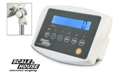
Very simple to use multifunction weight indicator in ABS. Connectable to load cell platforms; pieces counting, % weight, weight check, totalisation/formulation functions. Internal resolution of 600.000 points. CE-M approval for legal for trade use.
