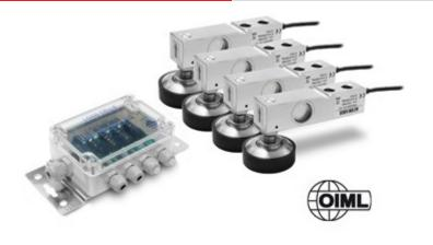
Ideal for creating platforms with 4 load cells of various sizes and capacities. The kit is made up of 4 1000 Ohm IP68 stainless steel load cells, OIML approved, together with adjustable stainless steel resting feet and an equalisation box.
