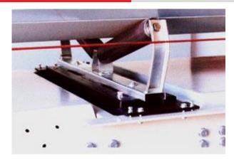
A single bar for continuous weighing, able to house one, two, or three rollers for a flat or concave conveyor belt. The module is suitable for creating continuous weighing systems, even for already existing ones. See also CPWEBELT
