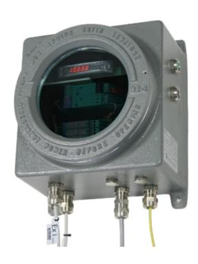
Box with Exd protection completed with weight indicator/transmitter, Zener barriers and intrinsically safe 4-20mA analog output. Fitted with 2 buttons for the main weighing operations with configurable functions, and two programmable electronic outputs for setpoints and levels management. Complete protection: ATEX II 2 (1) GD Ex d [ia Ga] IIC T6 Gb / Ex tb [ia Da] IIIC T85°C Db IP66.
