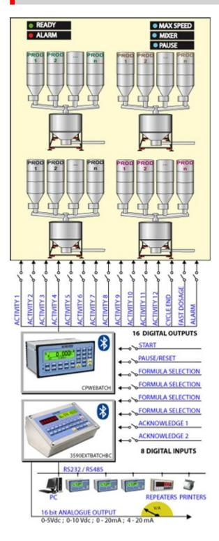
Software for multicomponent dosage with various scales, for CPWE and 3590EXT indicators.
