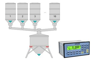
3590EXT and CPWE weight indicators software version for automatic multicomponent and multi scale dosage systems. Database of 100 different activities and 500 formulas.
