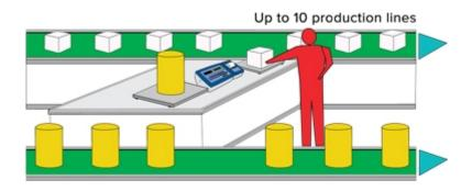
Suitable for advanced statistical checking applications of prepacked goods with data and print management (as provided for by the directive N. 76/211/EEC). Up to 5 independents connectable scales. CE-M approvable (OIML R-76 / EN 45501).
