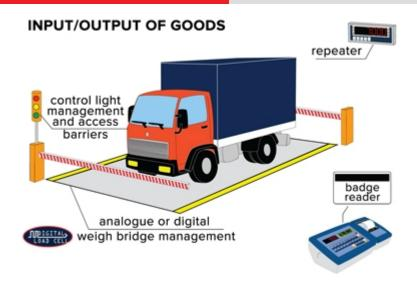
Particularly suitable for vehicle weighing and weighbridge management, with input/output control of goods. The AF03 version allows to weigh the vehicle by itself or with the trailer, either with the operator as well as self-service with the badge reader, as well as the advanced management of the data and the printouts. The AF03 also offers the possibility of managing the main digital load cells available on the market. CE-M approvable (OIML R-76 / EN 45501).
