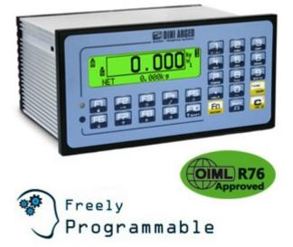
Multifunctional microcontroller/ weight indicator for use in industrial systems. 16 outputs and 8 digital inputs, 3 RS232/RS485 serial outputs, 16 bit analogue output, Sysway transmission protocols and RTU Modbus are some of the features of this indicator, which, added to the range of available application software programs, allow the use in dosage and weight verification applications, with direct management of the automation. CE-M approvable (OIML R-76 / EN 45501).
