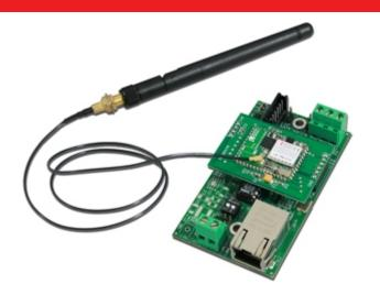
Small size, excellent signal quality and adjustment of the antenna's inclination and orientation, are just a few features of this product which allow for an easy wireless connection of any scale or weighing system to the company's computer system; it' easy to install and it's fitted with a cable for the connection to the indicators.
