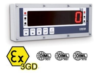
Weight indicator/ repeater particularly suitable for use in hazardous environments, where it's necessary to view the weight from a distance at any angle. Usable in areas: ATEX II 3G Ex nR IIC T6 Gc X for gases ATEX II 3D Ex tc IIIC T85°C Dc IP68 X for dust. Fitted with a very bright 60mm LED matrix display and IP68 stainless steel case. CE-M approvable (OIML R-76 / EN 45501).
