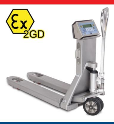
Pallet truck scales, with built-in electronic weighing, for dangerous areas classified as hazardous (ZONES 1 and 21 & 2 and 22) in accordance with Ex II 2GD IIB T4 T197°C X. The weight detection made with four Atex certified IP68 stainless steel load cells guarantees the best precision in any working environment.
