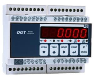
Multipurpose weight transmitter for panel mounting on DIN bar. Ideal as an independent or dependent 4-channel digital junction box, permitting the direct reading and diagnostics of each connected load cell. The wide range of available interfaces, makes it easy to integrate the weighing with any automation system. CE-M approvable (OIML R-76 / EN 45501).
