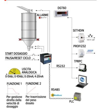
Example of dosage system for discharging with the DGTQF
