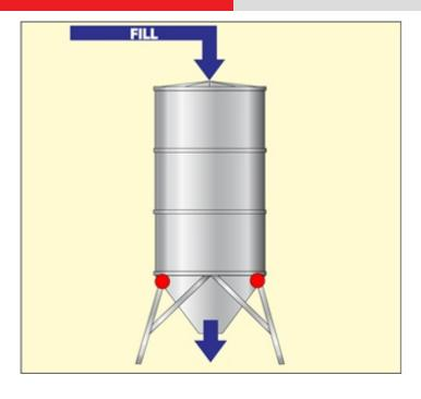
Configuration which allows to manage a dosage system in unloading of a single product, useful for dividing the quantity of materials of equal weight or extract precise quantities from the silo, with management of the reloading.
